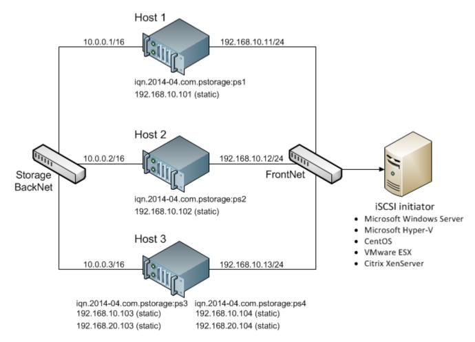
In this example are three Virtuozzo Hardware Nodes working in a Virtuozzo Storage cluster. Two Nodes host one iSCSI target each while the third hosts two iSCSI targets. Each Node has a static or dynamic IP address assigned from the Storage BackNet (created along with the Virtuozzo Storage cluster) and the FrontNet. Each iSCSI target has a static IP address assigned from the FrontNet.
