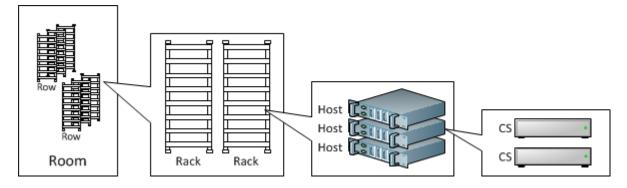
The first 3 topology path components, room.row.rack, can be configured in the /etc/vstorage/location configuration files (for more information, see the man page for vstorage-config-files). The last 2 components, host\_ID.cs\_ID, are generated automatically:
